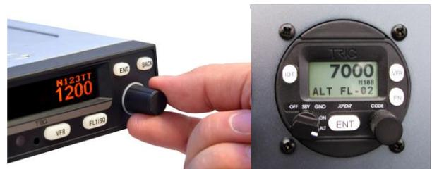
Both models are ADS-B Out capable. The TT21 is designed to fit in the tightest panel space. This transponder has an 130 Watt output and uses an external antenna - so your aircraft is visible at all times. Trig transponders meet the latest regulatory standard, ETSO-C166b.
